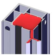
Apply sealant to each end of the True Divided Light post as shown above.
