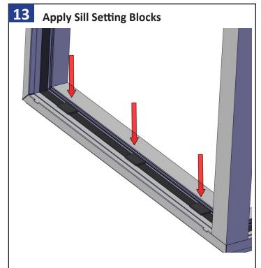
Insert provided setting blocks on the sill. Place 1 block in each corner no more than 2" from the jamb or TDL post. Continue to place blocks along the sill spacing them no more than 18" apart.
