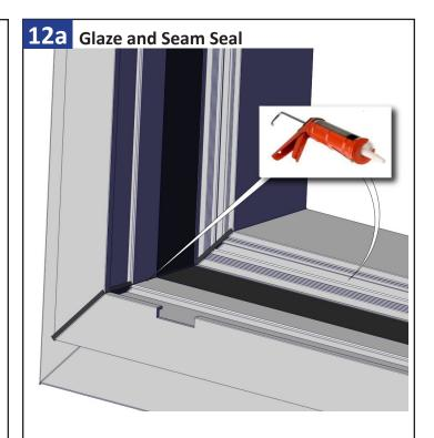
Apply a continuous 1/4" bead of sealant along the glazing legs filling the T-track. Then apply a bead of sealant along the inside corners of the frame from the glazing leg out to seal the seam. Tool the sealant in the corners.
