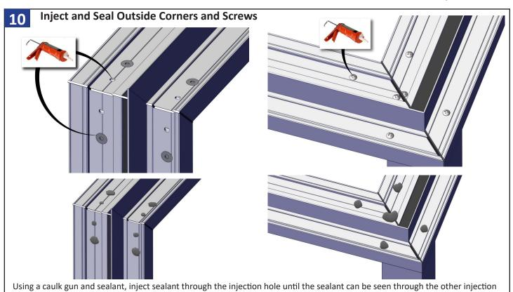
hole along that corner key. Fill all injection holes. Also completely cover the screw heads for all corner key screws. Repeat for
