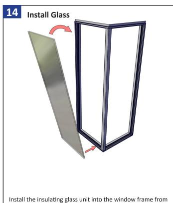
the exterior, bottom first and tilting the glass into the frame.
