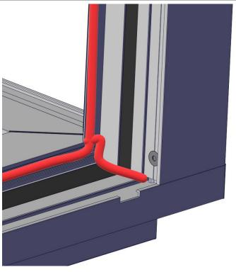
Sealant applied to glazing legs and inside corner of TDL. Repeat for corner at the head.
