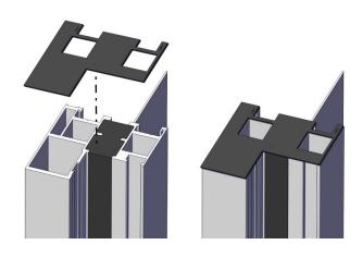
Attach a gasket to each mitered end of the jambs. Each jambs gets 2 gaskets.
